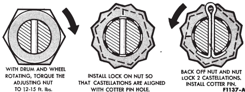
FIG. 4—Front Wheel Bearing Adjustment
